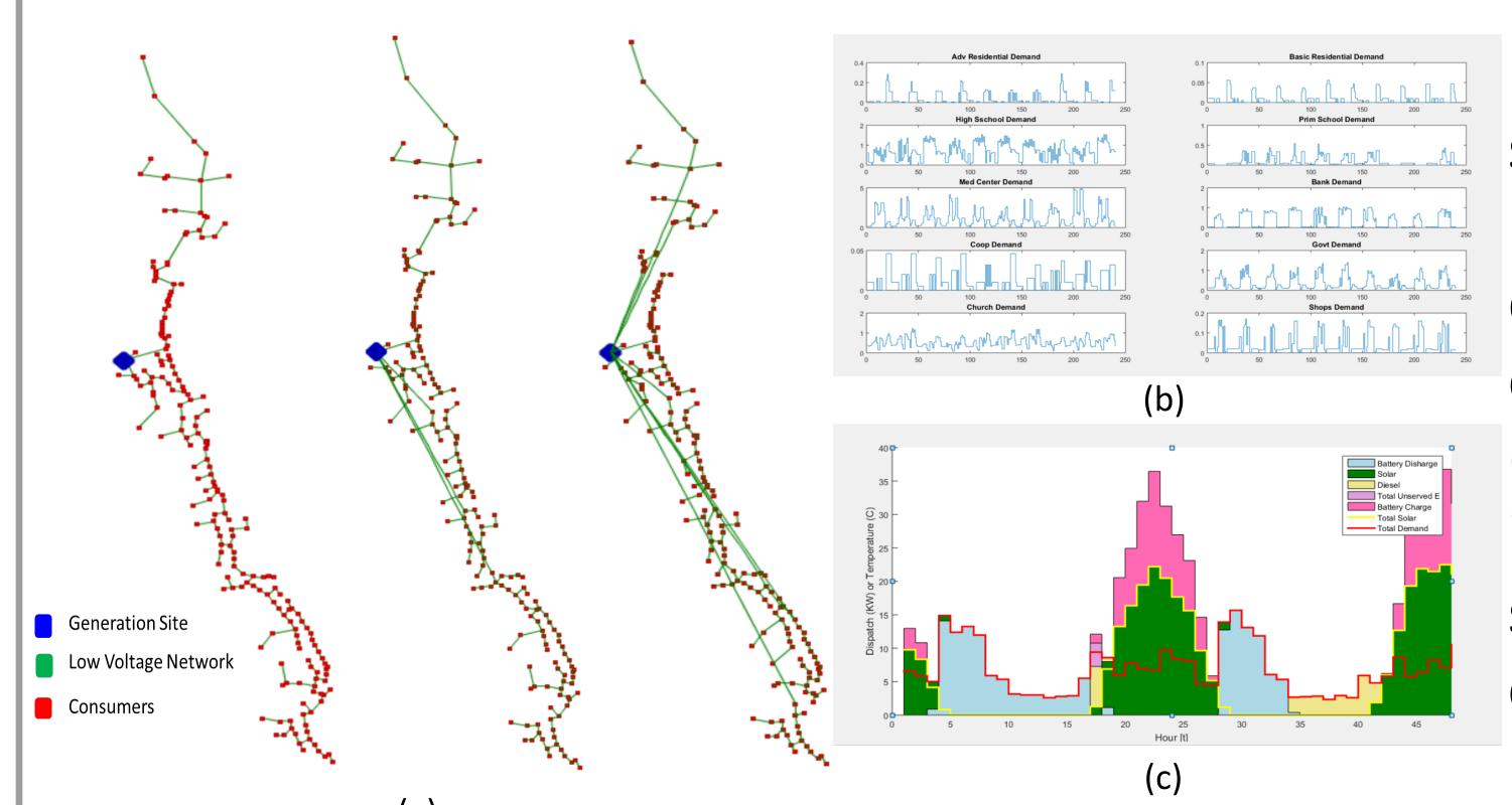
Detailed microgrid system designs are proposed (a) based on demand profiles for different user types (b), time varying solar irradiance data, and sample dispatch calculations (c).
