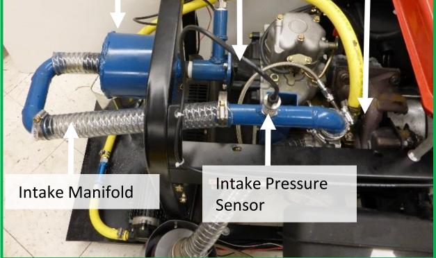
Simple experiment built to test the first order feasibility of turbocharging a single cylinder diesel engine.
